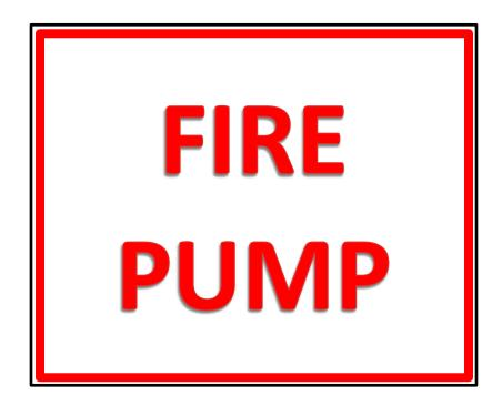
Minimum Size: 5" x 7" Lettering: Red lettering on white background with solid red border Installation: Post on the exterior of the door to the room where the Fire Pump is located
